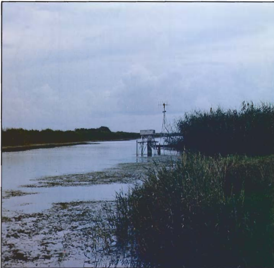
Collected data is sent by VHF signal from remote station 1-8C to the base station at Clewiston. A total of 10 such stations monitor water level and rainfall in water conservation areas of the Everglades.
