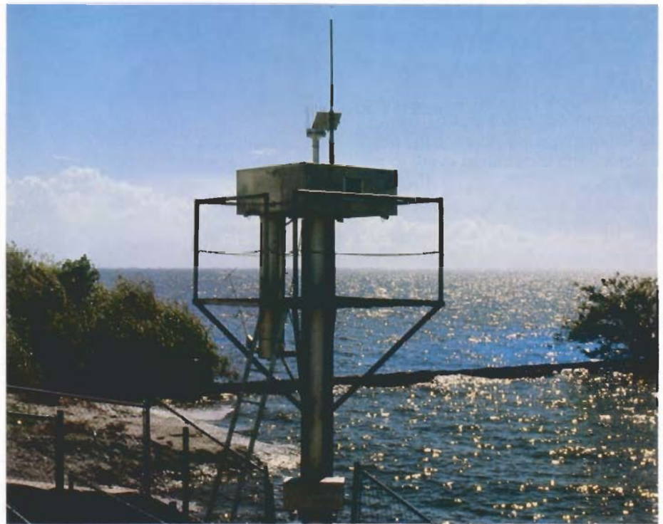
Water level and rainfall data is collected on Lake Okeechobee by the Port Mayaca remote automatic platform, one of four which send data by satellite to locations in four states.
